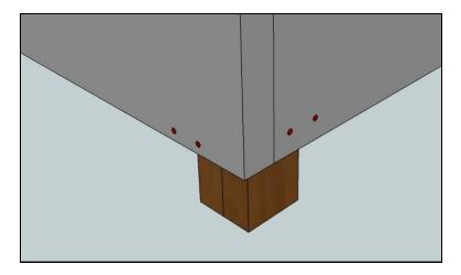
**Step 7:** Attach the legs to the corners of the bed frame as shown using pocket hole screws or wood screws.
