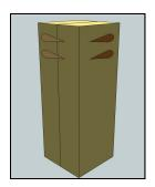
Otherwise, drill four (4) pilot holes in each corner as indicated. The holes are offset so the screws do not interfere with each other.
