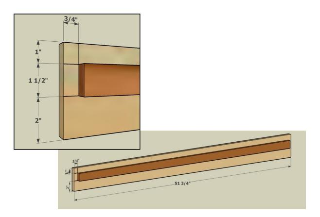
**Step 3**: Cut two (2) Head/Footboard A from 1x6 stock. Cut two (2) Head/Footboard Bs from 1x2 stuck. Spread wood glue onto Head/Footboard B. Nail Head/Footboard B to Head/Footboard B as shown.
