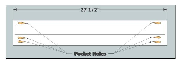
Otherwise, drill six pilot holes as indicated into your Side Rail assemblies. Use a countersink to create a finished look.
